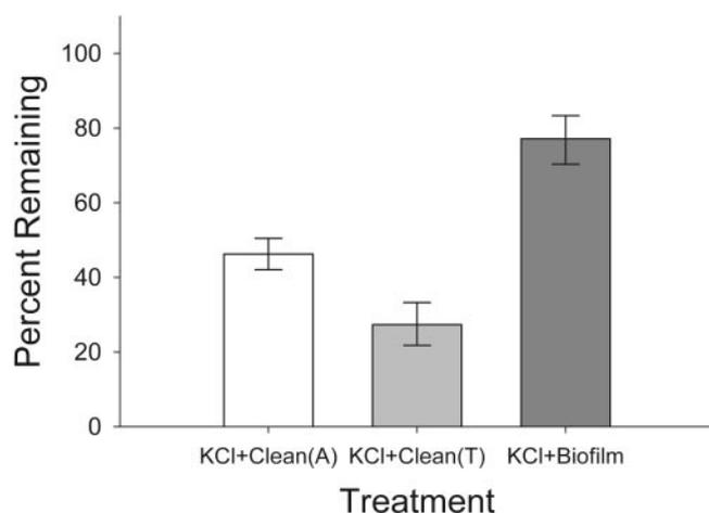
**Figure 2.** Mean percentage of *Phallusia nigra* remaining on slides after exposure to a nominal wall-shear stress of 120 Pa. Treatments consisted of glass slides cleaned with acid (A) or Triton X-100 (T), or coated with a natural biofilm. Excess KCl ( $10 \text{ mmol l}^{-1}$ ) was applied to all treatments. Error bars = 1 SE.
