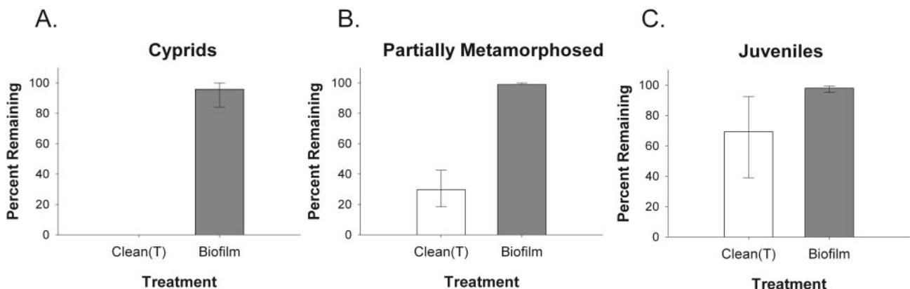
**Figure 4.** Mean percentage of *Balanus amphitrite* remaining on slides after exposure of a nominal wall-shear stress of 120 Pa. Metamorphosed individuals were evaluated at the (A) attached cyprid, (B) partially metamorphosed, and (C) post-metamorphic juvenile stages. Treatments consisted of glass slides cleaned with Triton X-100 (T) and biofilmed slides. Error bars = 1 SE.
